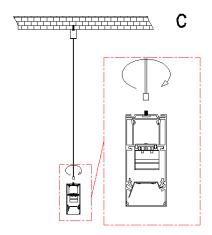
A. fix metal canopy with screws on ceiling.
