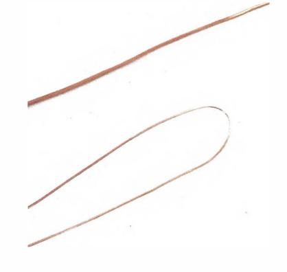
Position the bent center of the weaving wire around the central point of the base wire, as shown here.
