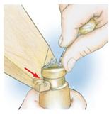
An 80 grit  $\frac{1}{2}$ " x  $\frac{1}{2}$ " abrasive band and mandrel (drum arbor) works well for this modification. Draw a reference line on the ring clamp about 10mm from the end. Use the abrasive band to create a two-millimeter indentation around the ring clamp. Test the groove against your bench pin(s) and make adjustments as necessary so the clamp locks in place.
