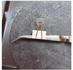
Small part sanding tip for sanding many tiny details. Use a sticky paper double sided tape. It holds loose pieces in place for easier sanding.
