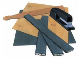
Essential bench tools, sanding sticks are used for finishing metal surfaces throughout the jewelry making process. Although some suppliers offer them, most bench jewelers make their own. Sanding sticks are used progressively from coarse to fine in preparation for buffing and polishing metal, and they are virtually indispensable for jewelry work.
