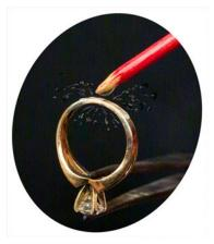
So try this the next time you need to re-apply flux to a hot piece of metal. Use the sharpened end of the brush to transport it. After removing the paint, which would burn upon contact with hot metal, dip the bare wood into flux to saturate it and transport it to the needed joint. The flux splatters of course, but it winds up in the right place without loosing a hair on your favorite brush
