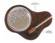
You've probably noticed an attractive pattern that looks like over lapping swirls on some machined metal surfaces. This is theresult of end milling, through which a series of circles can cover a surface evenly and uniformly. While jewelers may not be able to replicate the machine precision of professional milling, alluring optical surfaces can be
