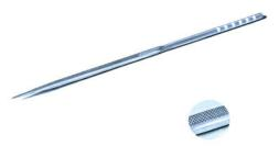
After rough grinding, take the file to an oiled sharpening stone-the kind you use to sharpen gravers, drill bits, blades, etc. Hold the file flat against the stone and rub it back and forth to smooth the new surface and remove marks left by grinding. When the surface is smooth, knock the cuts off the edges on both sides of the newly cleaned surface.
