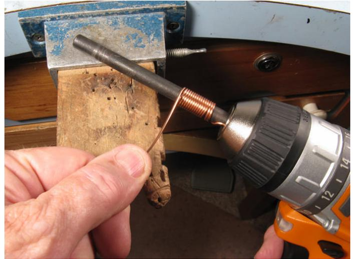
To wind a coil, just bend a right angle on the end of the wire about a half inch long and insert this into the screw gun chuck. Then wind slowly, keeping a tight coil. I like to rest the end of the mandrel on the edge of the table or bench pin. Finally, one note of caution. If you are winding an entire length of wire, be careful as you get near the end of the wire. If the end passes under your thumb, it can cause a nasty scratch or cut.
