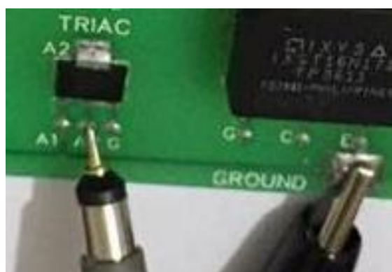
Figure 168: Channel1 Probe Used for Anode2 - Anode1 Measurement
