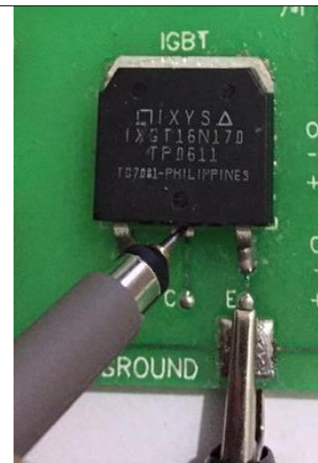
Figure 151: Channel1 Probe Used for Collector - Emitter Measurement
