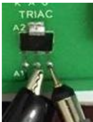
Figure 166: Channel1 Probe Used for Gate - Anode2 Measurement
