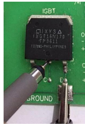
Figure 147: Channel1 Probe Used for Collector - Emitter Measurement
