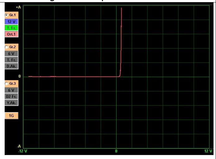
Figure 63: Diode VI Curve
