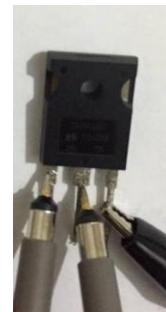
Figure 142: Sample of a Defective N Channel FET
