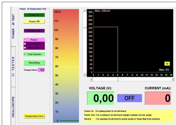
Figure 41: Adjusting the Voltage and Current (Step 1)
