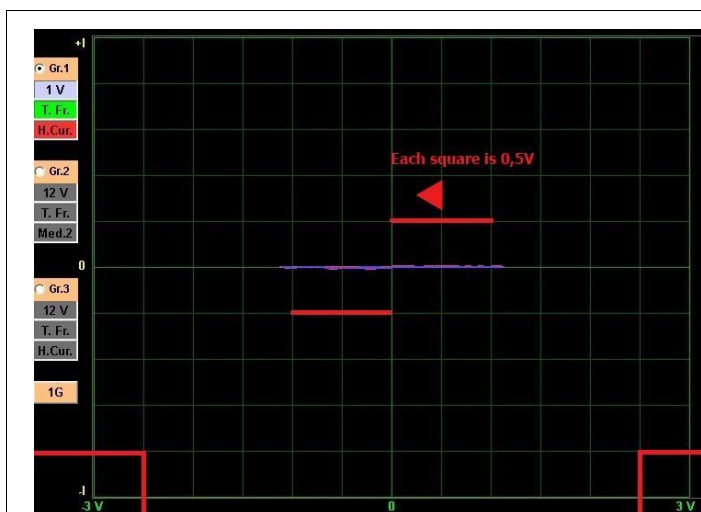
Figure 55: If the Test Voltage 1V, Each Square Represents 0,5V.
