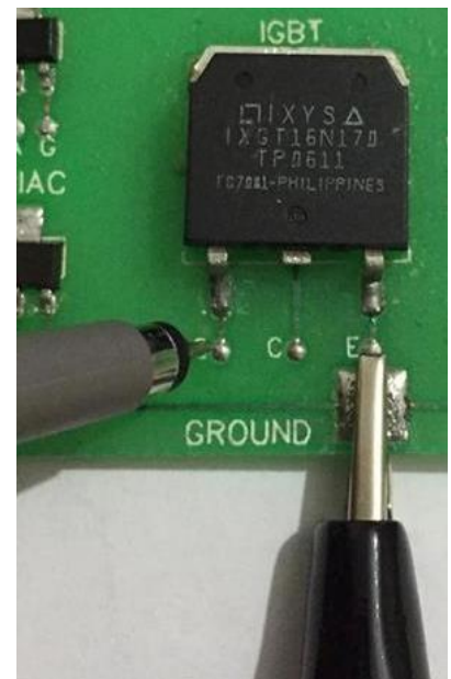
Figure 145: Channel1 Probe Used for Gate - Emitter Measurement
