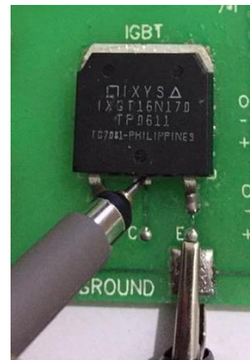
Figure 149: Channel1 Probe Used for Collector - Emitter Measurement
