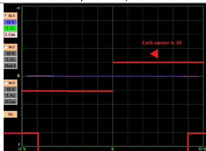
Figure 58 : If the Test Voltage 12V, Each Square Represents 2V.
