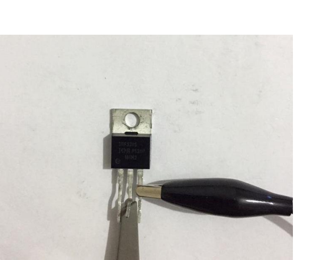
Figure 133: Channel1 Probe Used for Drain - Source Measurement
