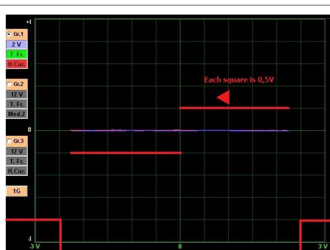
Figure 56: If the Test Voltage 2V, Each Square Represents 0,5V.
