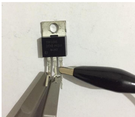
Figure 134: Channel1 (+), Channel2 (+), COM (-) Transistor Test
