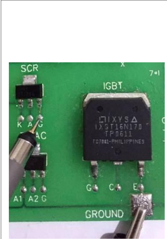
Figure 155: Channel1 Probe Used for Gate - Cathode Measurement
