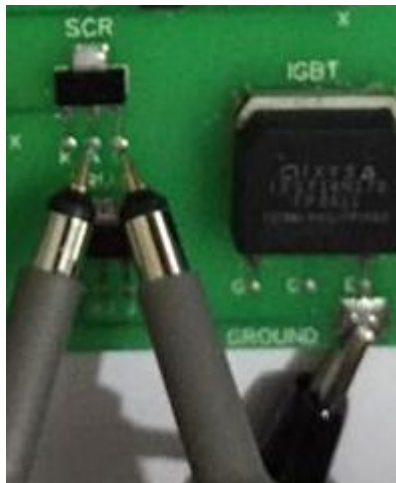
Figure 161: Channel1 (+), Channel2 (+), COM (-) Thyristor Test
