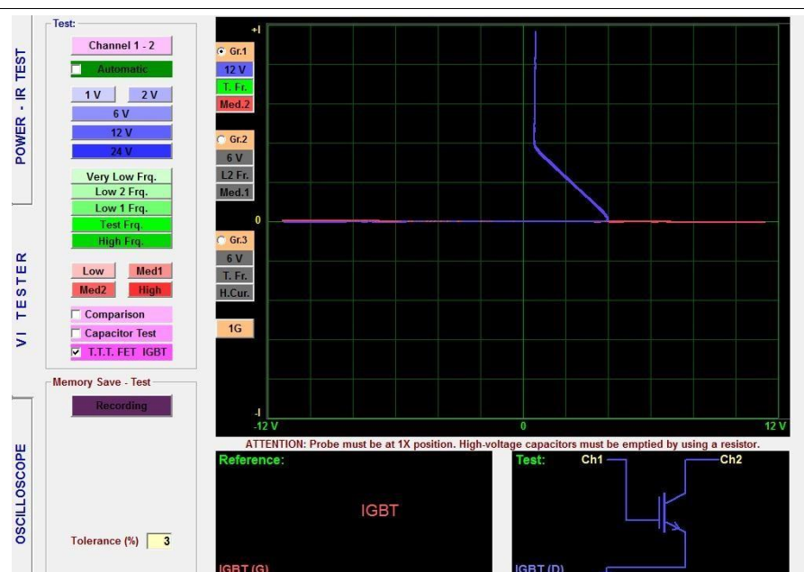
Figure 153: IGBT VI Graph, Equivalent Circuit Diagram
