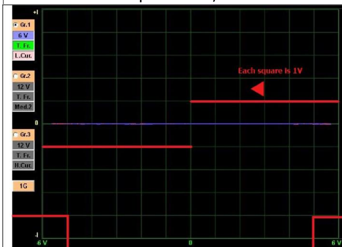
Figure 57 : If the Test Voltage 6V, Each Square Represents 1V.
