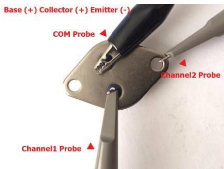
Figure 111: Channel1 (+), Channel2 (+), COM (-) Transistor Test
