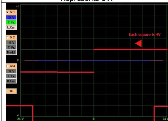
Figure 57 : If the Test Voltage 6V, Each Square Represents 1V.
