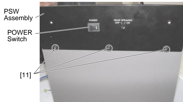
[11]: Bind Head Tapping Screw-1 3.5X12 MFZN2BL (EP030340) (Photo. 59)
