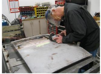
Photo #4 We removed the door to put a new door skin on.
