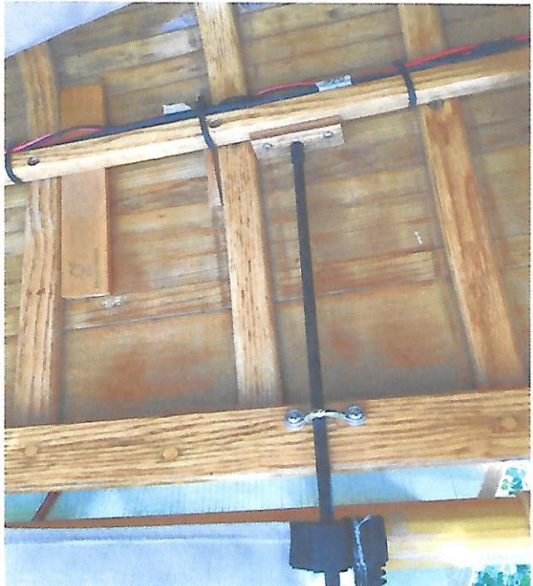
Figure 23. View showing how graphite tent supports were attached to boat.
