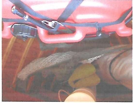
Figure 19: View of net-shelf fitted under deck supporting tent, rod container, folding chair, etc..
