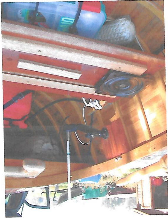
Figure 12: Swivel seat, rails, and seat lock.
