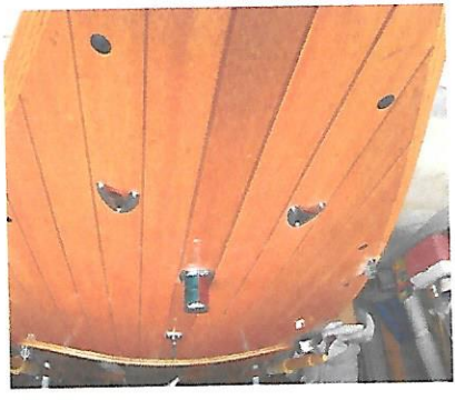
Figure 9. Twin vents in deck.
