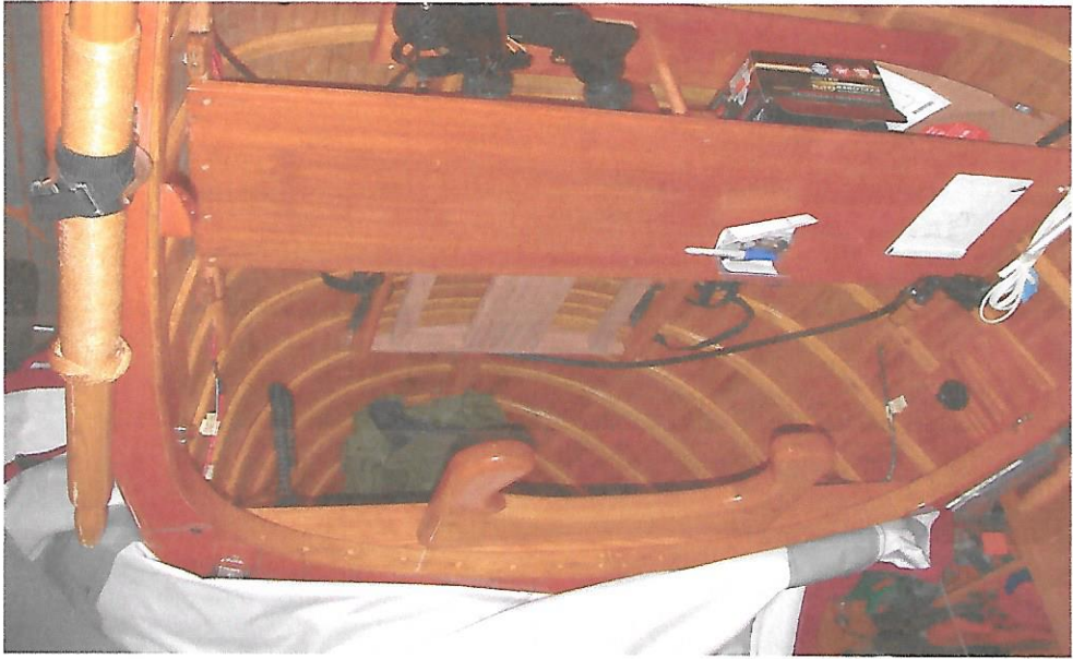
Figure 10: View of yoke, cradle for fuel tank, dowel, and oar.
