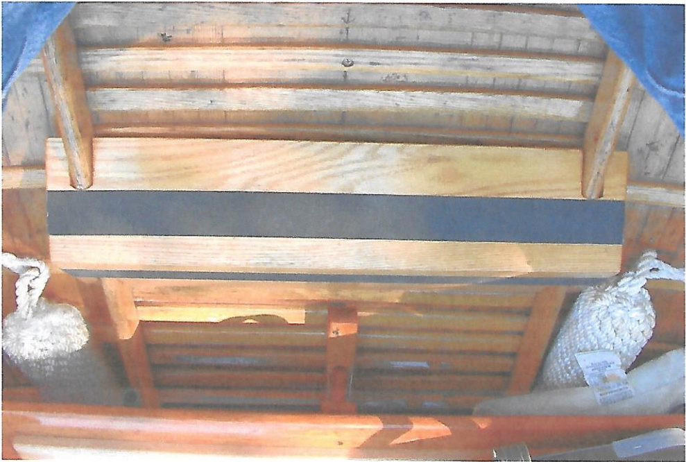
Figure 9: View of mobile foot rest mounted on rails.
