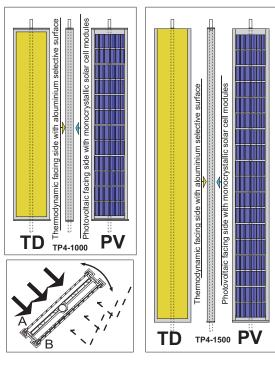
The twin faced TP4-Multipanel TD/PV/PVT can be rotated 360' around its central pipe, exposing either the main facing side (A) 'thermodynamic mode', or the other facing side (B) 'photovoltaic' mode towards the solar radiation. Both sides are
