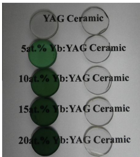
Fig. 1. Photos of YAG transparent ceramics doped with 0, 5 at.%, 10 at.%, 15 at.% and 20 at.% Yb concentration (left denotes pre-annealed samples and right denotes post-annealed samples).
