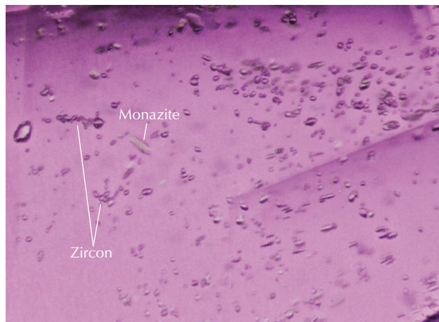
Figure 94. A series of colorless zircon inclusions and orange-brown monazite inclusions in the heated purplish pink sapphire. Photomicrograph by Ugo Hennebois; field of view 1.5 mm.
