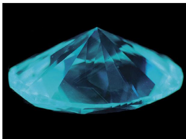
Figure 87. Deep-UV imaging of the 0.71 ct colorless diamond showing a cuboctahedral-structured luminescence associated with HPHT growth. Image by Guy Borenstein.
