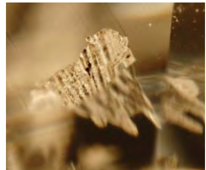
Figure 19. Dark, rounded grooves along the length of this cavity in the 8.38 ct diamond are further indications of laser drilling. Magnified 45x.
