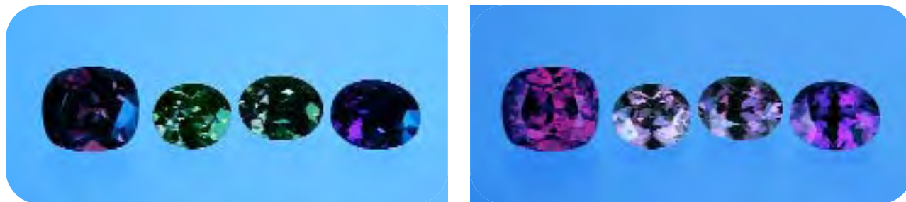
Figure 10. Chemical differences (table 1) are responsible for the different colors shown by the pyrope-spessartines from Tranoroa as compared to pyrope-spessartines from Bekily in day or fluorescent light (left) and incandescent light (right). From left to right: sample E, 2.02 ct from Tranoroa, with Cr>V; sample X, 0.67 ct from Bekily, with V>Cr; sample Y, 0.90 ct from Bekily, with V~Cr; and sample Z, 0.78 ct from Bekily, with V>Cr. Photos by Maha Tannous.
