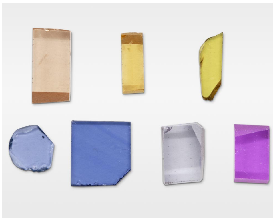
Figure 2. Shown are some of the many crystallographically oriented samples used in this study. Clockwise from top left, they represent the following chromophores: h^{\bullet}\text{-Cr}^{3+} , h^{\bullet}\text{-Fe}^{3+} , \text{Fe}^{3+} , \text{Cr}^{3+} , \text{V}^{3+} , and \text{Fe}^{2+}\text{-Ti}^{4+} (the two blue samples at lower left). The sample in the far lower left corner is a natural blue sapphire from Yogo Gulch, Montana, and the sample in the upper right corner is a natural yellow sapphire from the Subera deposit in Queensland, Australia; the rest are Czochralski grown. Sample numbers clockwise from upper left are 991, 992, 1121, 1110, 1102, 1065, and 1014; detailed information on the samples can be found in Appendix 1.
