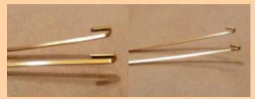
together at three points that will wrap tightly around your cab. The short pieces of 1/2 round wire will hold the square wires together. Pick up one piece of 1/2 round wire and use the flat nose pliers to bend 3-4 mm of the top over. Then angle the bend slightly. Make sure the flat side of the wire is on the inside surface. This will fit neatly around the square wire.
