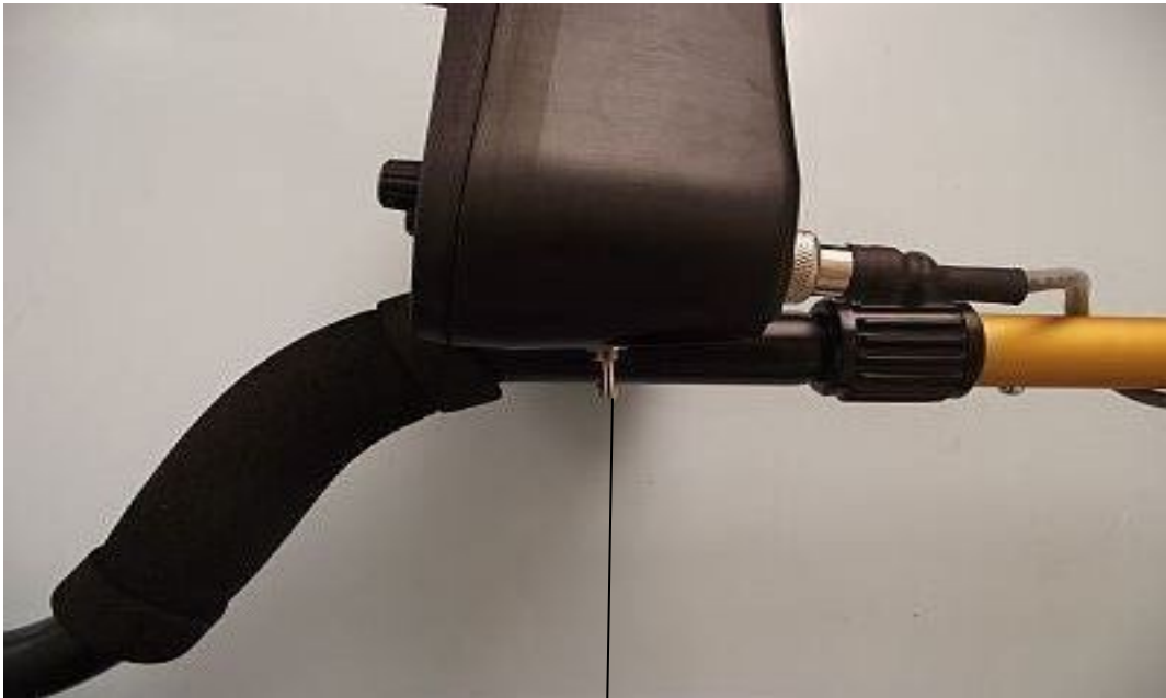
THREE POSITION TRIGGER SWITCH (MIDDLE POSITION) ALL METAL MODE
