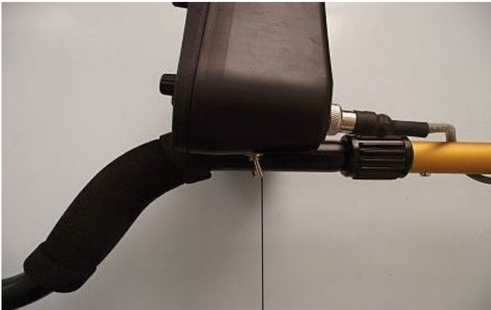
THREE POSITION TRIGGER SWITCH FORWARD POSITION (Trigger pushed furthest from you.) 2-TONE MODE
