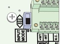
Use the following instructions to electrically connect the input channels in parallel.
