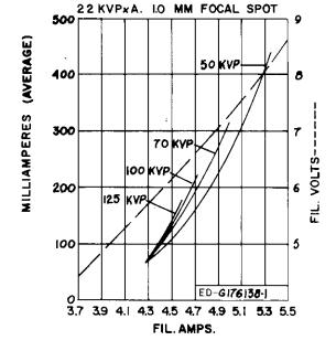
MAX. CONTINUOUS CURRENT 3.30 AMPS. MAX. ALLOWABLE CURRENT 5.50 AMPS.
