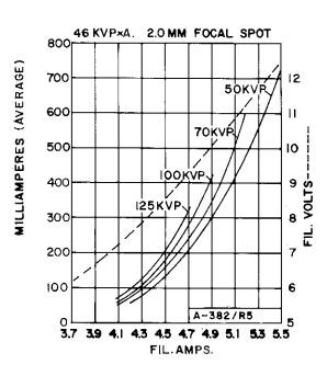
MAX. CONTINUOUS CURRENT 3.30 AMPS. MAX. ALLOWABLE CURRENT 5.50 AMPS.
