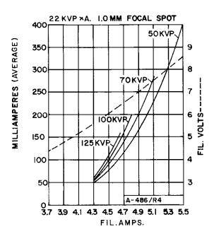
MAX. CONTINUOUS CURRENT 3.30 AMPS. MAX. ALLOWABLE CURRENT 5.50 AMPS.
