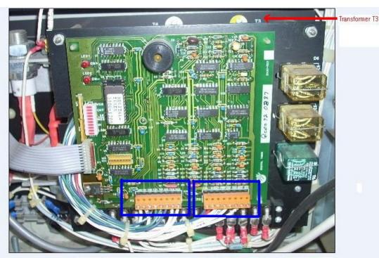
Check all the wire connections at connectors P2 and P3. Check that the wire is bare going into each screw terminal connector of P2 & P3. Check that all the screw connections are tight on P2 & P3
