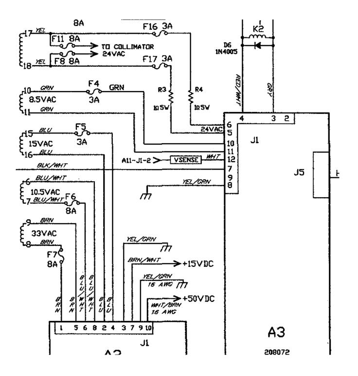
If the fuses are good and you still don't have 24 vac to the micro, check if either or both of these resistors are open.
