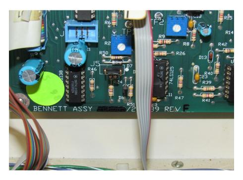
J5 jumper is on the middle two pins for anode selection
