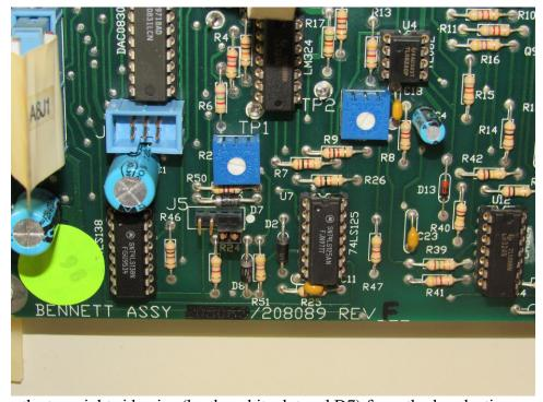
J5 jumper is on the two right side pins (by the white dot and D7) for cathode selection
