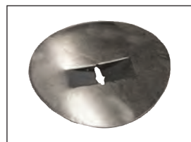
Metal 15/16 No. 15 Spring Washer. Made of precision tempered spring steel. Prong is forced through opening and locked by spring action.
