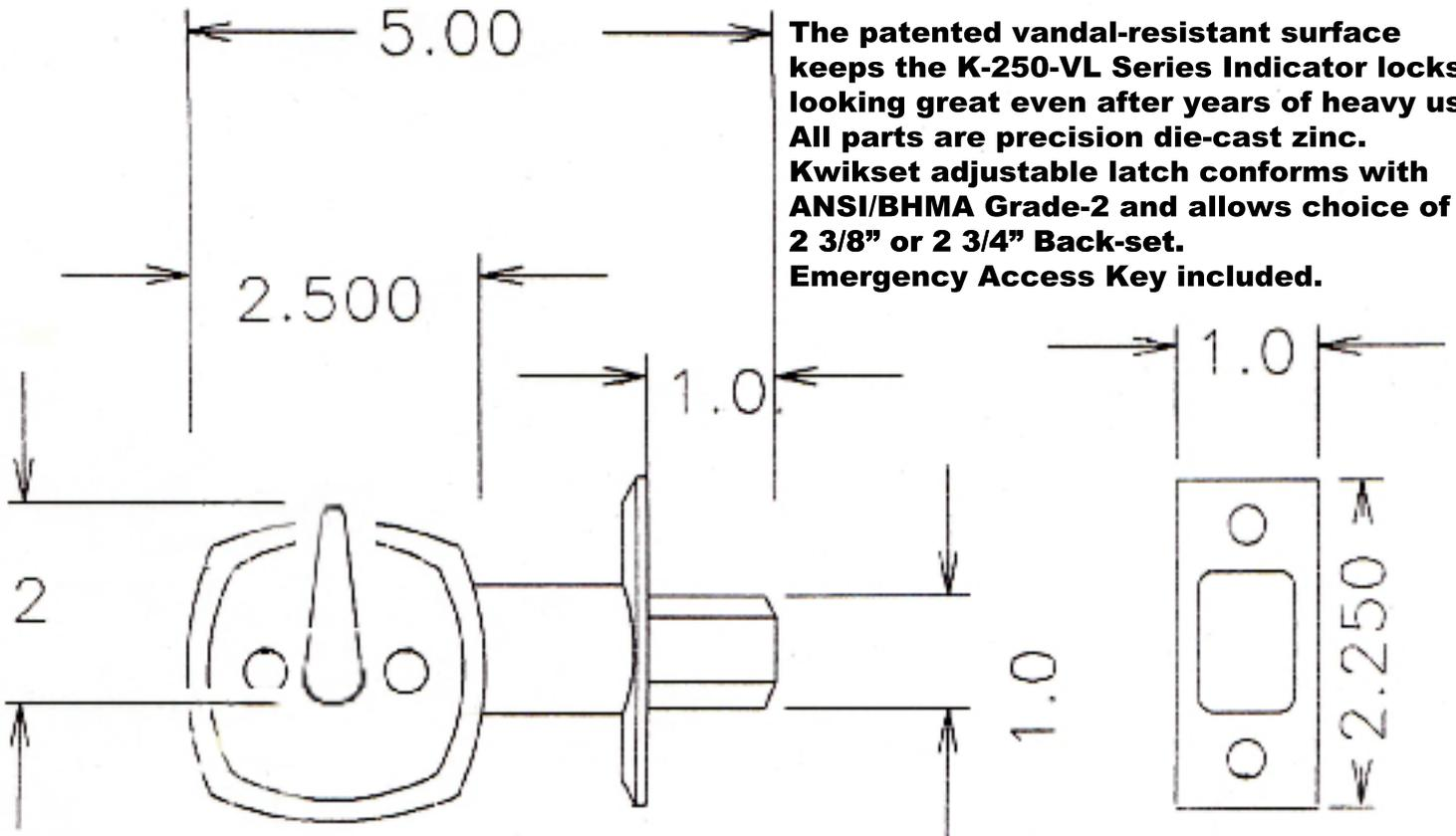
The patented vandal-resistant surface keeps the K-250-VL Series Indicator locks looking great even after years of heavy use. All parts are precision die-cast zinc. Kwikset adjustable latch conforms with ANSI/BHMA Grade-2 and allows choice of 2 3/8" or 2 3/4" Back-set. Emergency Access Key included.
