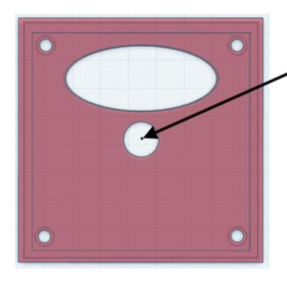
Place this template onto the outside of the door, aligning the large center hole with the 1/2" hole you drilled through from the inside.
