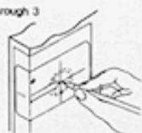
B. Drill 1/8" (3mm) diameter pilot holes where marked.
