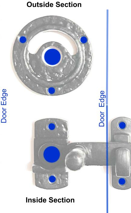
2 Drill the two small holes for a #6 screw size.
