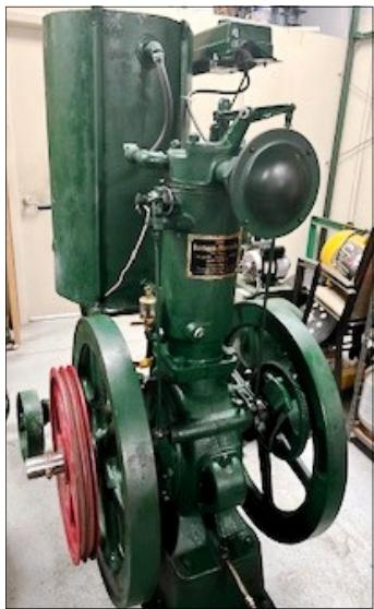
engine was locked up when he originally got it and he set about trying to free it. It took six months with a chain he attached a weighted cheater bar until the fly wheel was finally freely moving.
