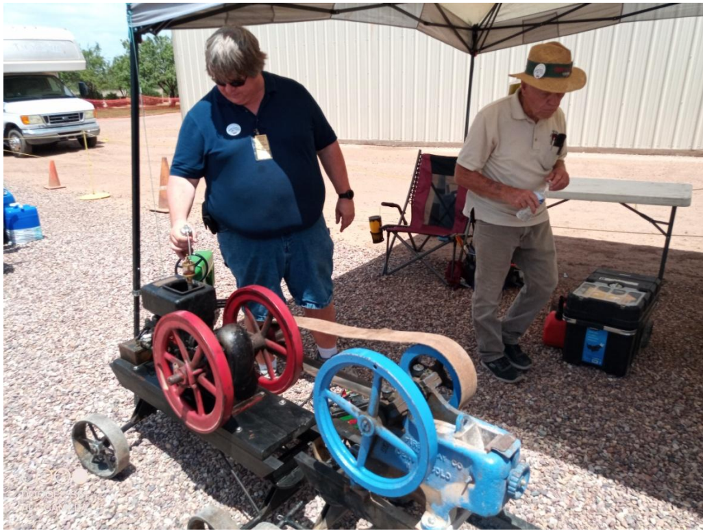
Lyle Showing Hit & Miss Engine With Rock Crusher
