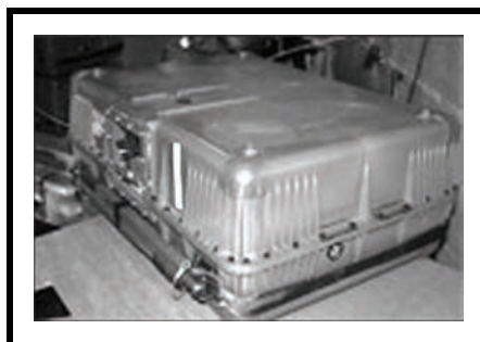
Figure 14-4. M-131 Modular Pack Mine System (MOPMS).
