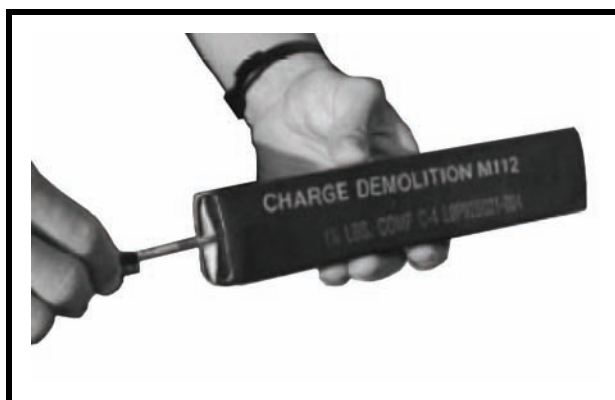
Figure 14-9. Priming of C4 demolition blocks with MDI.
