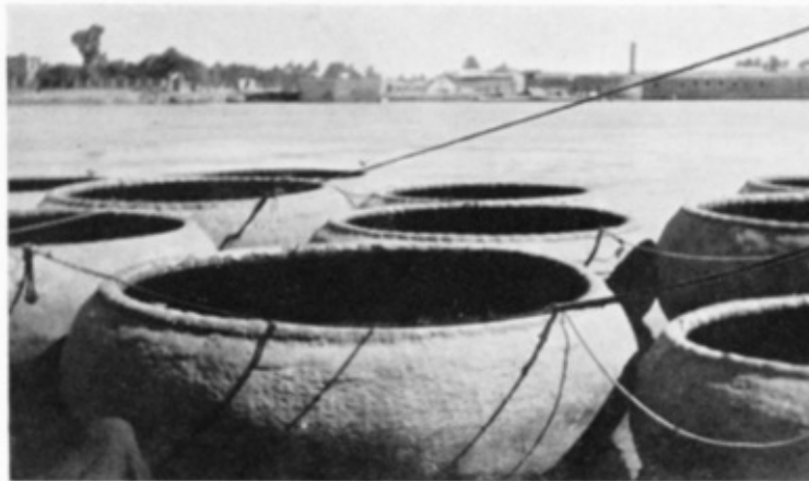
(3). The finished gufa, daubed with bitumen to make it watertight.
