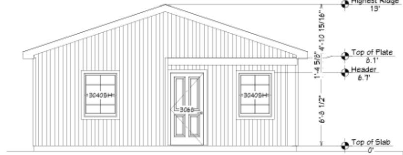
Exterior Elevation Front
