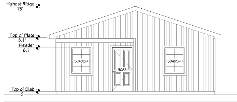
Exterior Elevation Front
