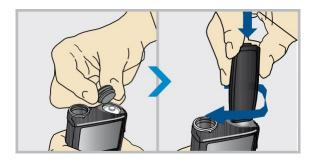
3. Place battery cap into the pump and use the edge of the belt clip to screw the cap back on.
