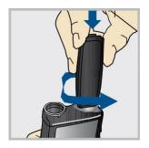
1. Unscrew the battery cap using the bottom edge of the belt clip. (Or use a thick coin.)
