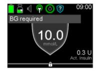
If the pump is in Safe Basal and there is something that can be done to resolve the issue, the pump will alert the student what to do, like check a BG.
