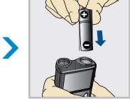
2. Insert battery with negative (flat) end going in first.
