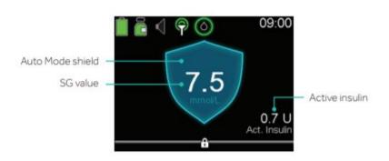
If you see the SmartGuard™ shield, the pump is in Auto Mode, which includes Safe Basal.
