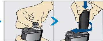
1.Unscrew the battery cap using the bottom edge of the belt clip. (Or use a thick coin.)
