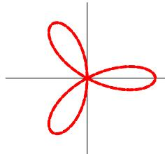
$$\begin{aligned} &= \int_0^{\frac{\pi}{6}} a^2 \cos^2 3\theta d\theta \\ &= a^2 \int_0^{\frac{\pi}{6}} \frac{1}{2} (\cos 6\theta + 1) d\theta \\ &= \frac{1}{2} a^2 \left[ \frac{1}{6} \sin 6\theta + \theta \right]_0^{\frac{\pi}{6}} \\ &= \frac{1}{2} a^2 \left( \frac{1}{6} \sin \pi + \frac{\pi}{6} - 0 \right) \\ &= \frac{1}{12} \pi a^2 \end{aligned}$$
