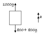
1000g - 800g - 800 = 800a 1200 = 800a a = 1.5For upward travel,  $v^2 = u^2 + 2as$   $= 0 + 2 \times 1.5 \times 1$  $v = \sqrt{3}$
