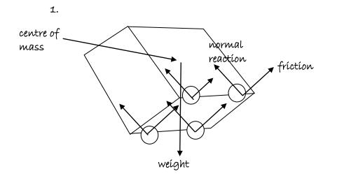
Normal reaction and friction forces act at the point of contact of each wheel
