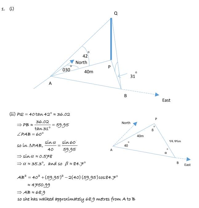
(iii) The bearing of the mast from B is approximately 324.7.
