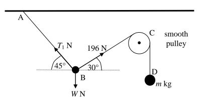
The diagram shows a load of weight W N at B in equilibrium. The load is attached by one light string to the ceiling at A and by a second light string that passes over a smooth pulley at C to an object of mass m kg hanging freely at D. The angles of the strings and the tensions  $T_1$  N and 196 N acting at B are shown in the diagram.
