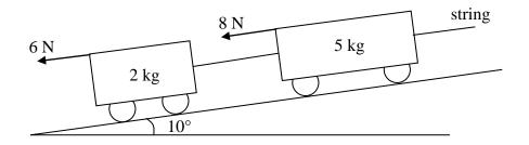
(i) In a case where the acceleration of the two trucks is 2.5 ms<sup>-2</sup>, show that the tension in the string is 43.4 N, correct to three significant figures.
