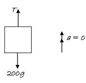
Since the lift is moving at constant velocity, the acceleration is 0. T - 200g = 0
