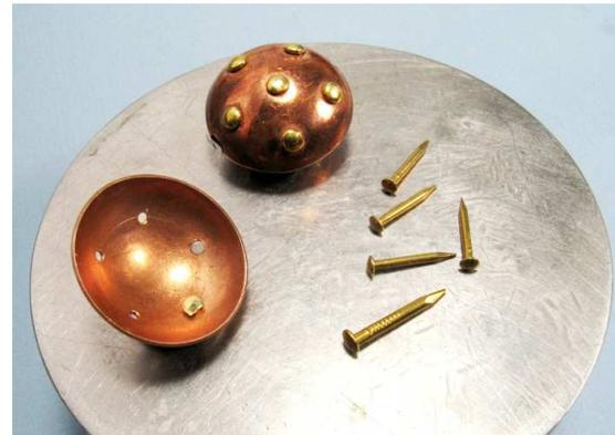
For best results, select a drill that gives you a hole with a close fit to the rivet. Trim the rivet to leave a little less than one diameter sticking out the back side. Place the head on a scrap of hard plastic on the anvil so as to not flatten the head. I prefer a ball peen hammer (with a small 3/8 inch ball) for setting the rivet.
