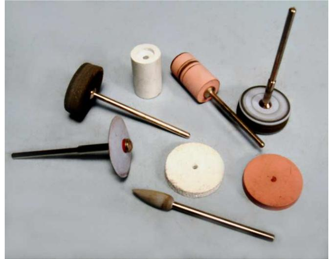
Cylinder shapes are nice for doing the inside of rings. Knife-edge shapes clean up the base of bezels quickly. Most jewelry catalogs carry these wheels, but often the color codes don't match between different manufacturers.
