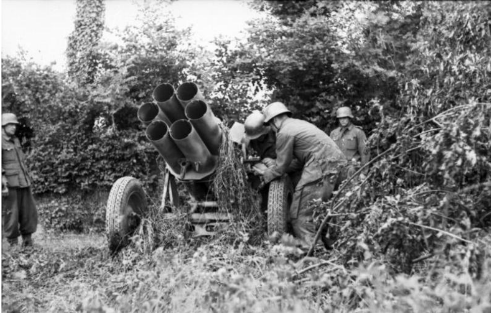
The 28/32 cm Nebelwerfer 41(NbW 41)was a six-barrelled rocket launcher mounted on a two-wheeled carriage.
